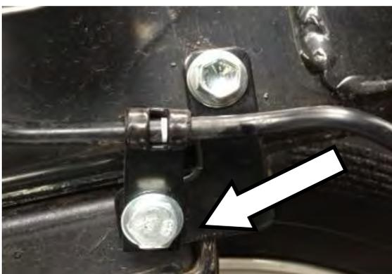
6. RE- ATTACH THE ORIGINAL HARD LINE BRACKET TO NEW OME BRACKET USING THE M8 BOLT AND WASHER PROVIDED. TIGHTEN ALL BOLTS THOROUGHLY.
