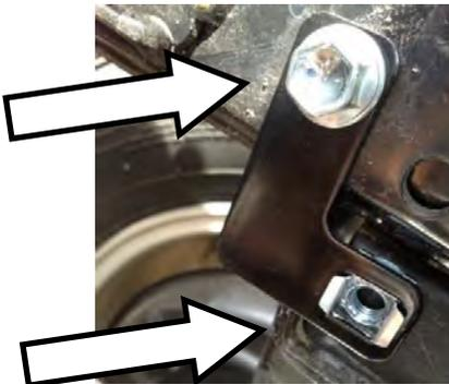
4. INSERT CAGE NUT INTO DROP BRACKET AND RE- USING THE ORIGINAL BOLTS, ATTACH TO THE CHASSIS
